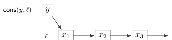
Figure 3: Structural sharing. Both lists exist; the new one reuses the old chain.
